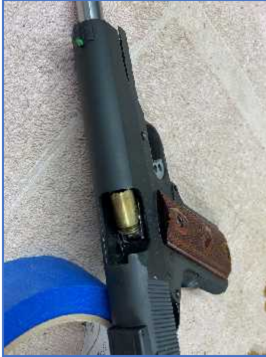
SRO with one of three stove pipes
