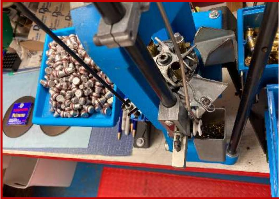
Looking down, am about eye level with my camera, you can see the handle, stage one, part of three, and stage four. The set up is ready for the handle to be pulled.<sup>2</sup>
