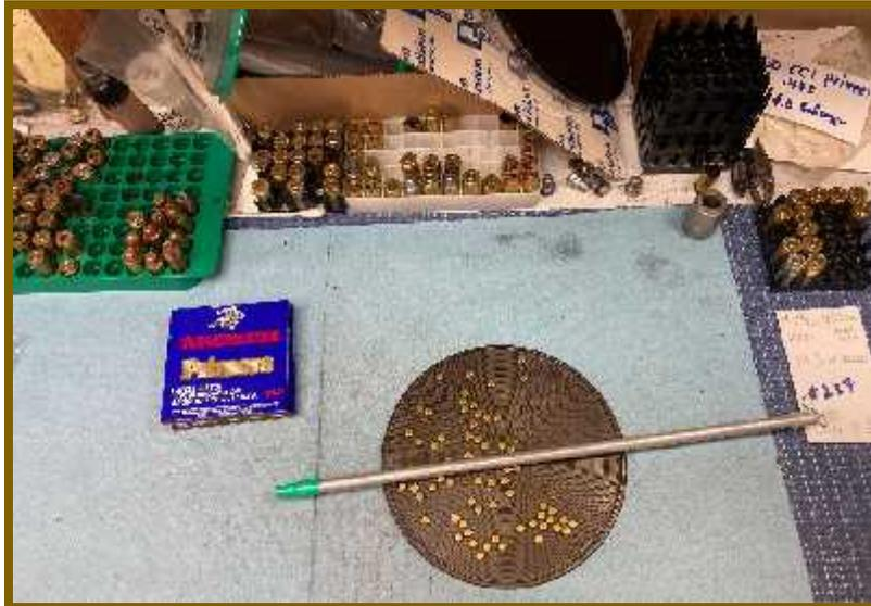
Shows half way through picking the primers up into the pick up tube. Note card for batch number 237 showing the date, recipe, and can number. The trays above the blue paper towels are holding mostly busted or broken brass, primers not working, or cartridges to be redone/fixed/discarded. I'd need six pages to explain all that but maybe whip up an appetite for some interest...meaning they don't always work and may mechanically fail.
