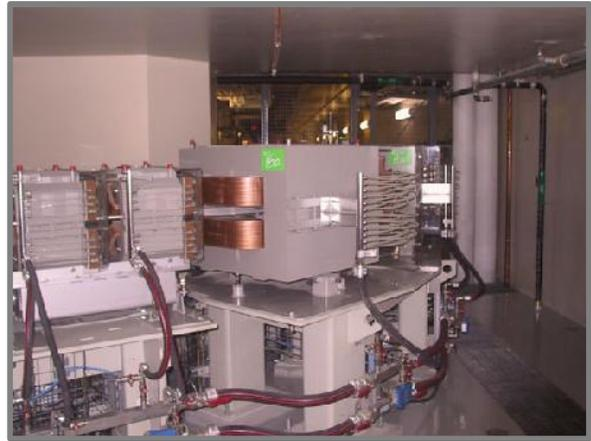
Beam pipe going north from cyclotron – then thru magnets and turning corner to the west to gantries.
