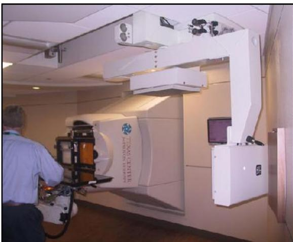
Inside Strength gantry (x-ray is on overhead rollers to the right).
