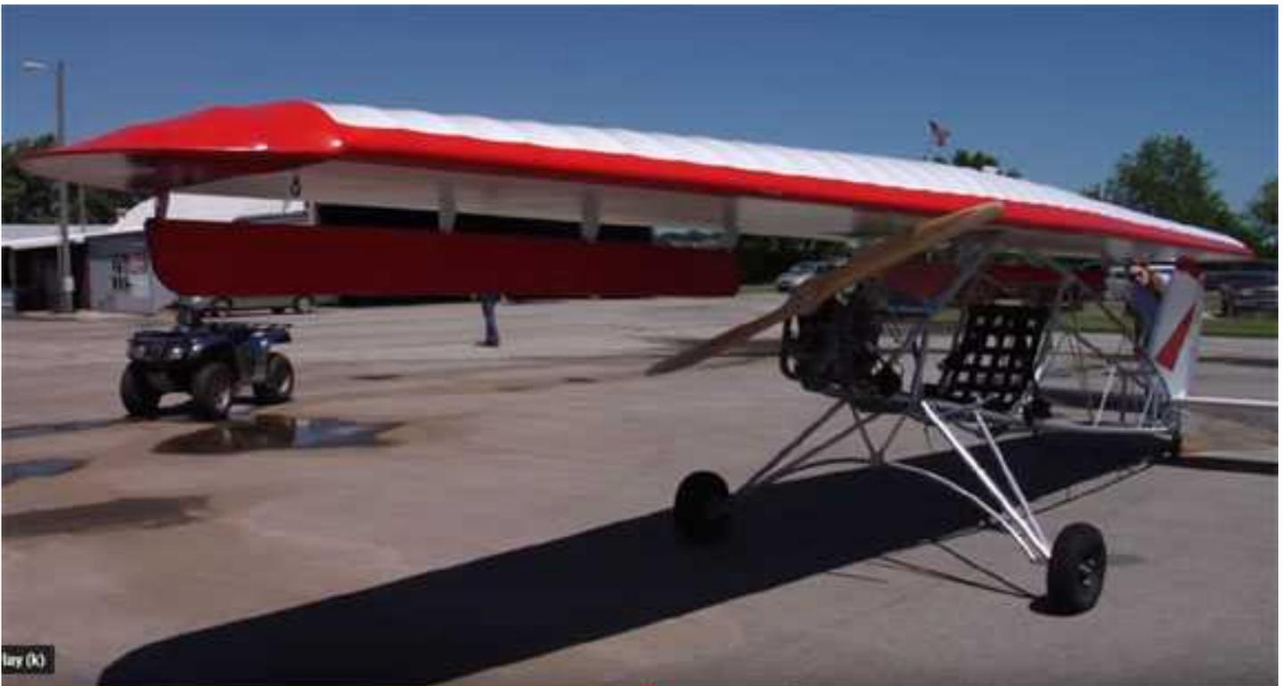
This is why it is called a swing wing. Needs a 30 foot trailer and away you go. Watch the video to see how they attach the wing to fuselage – and then watch how they hook up the ailerons. Is it failsafe and simple?
