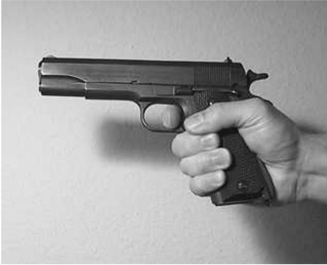
**HALF-COCK TEST:** Using thumb, pull hammer back until the first audible click. Hammer should be at half-cock notch. Grip gun normally, attempt to pull trigger. Hammer should NOT fall for any reason, unless the gun is a Series 80 commercial. These guns have a re-designed half-cock notch that engages near the at-rest position, thus the hammer cannot fall hard enough to strike the firing pin with force.
