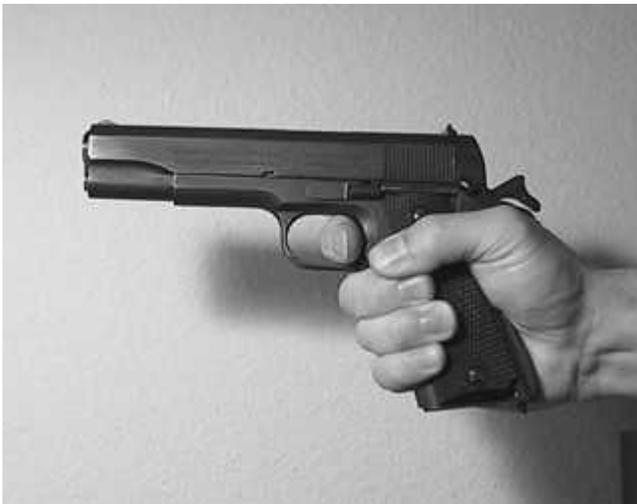
**THUMB SAFETY CHECK:** Holding gun normally with firing hand, slide forward, hammer cocked, thumb safety ON. Attempt to pull trigger. The hammer should not fall, nor should you feel any perceptible movement of internal parts. If you squeezed the trigger and it didn't come to a quick, hard stop (i.e. the trigger felt mushy) then there may have been some sear movement.
