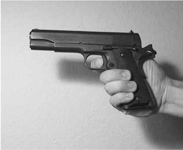
GRIP SAFETY TEST: Hammer cocked, slide forward, thumb safety OFF. Hold the gun so as to not depress the grip safety. Attempt to pull trigger. Hammer should not fall. If it does the grip safety is worn or has been deactivated.
