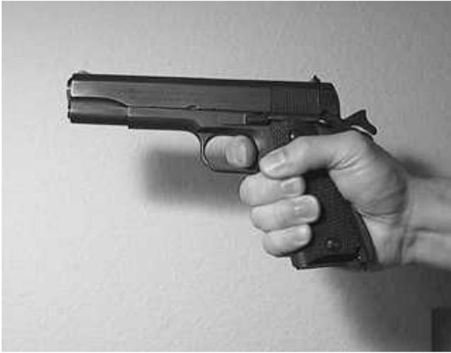
BASIC TEST: Slide forward, hammer cocked, thumb safety off, holding pistol normally with firing hand. Pull trigger-hammer should fall.
