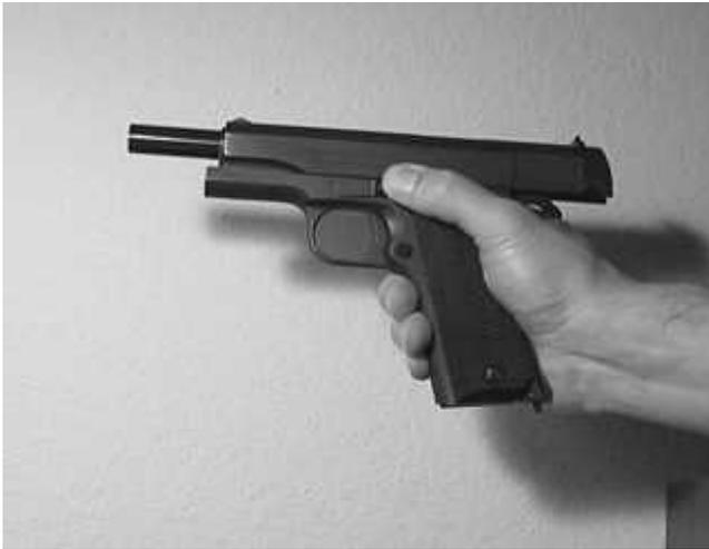
**SEAR ENGAGEMENT TEST:** Lock the slide back, grip gun normally, then release the slide stop, allowing slide to slam home with force. The hammer should NOT fall for any reason. If it does then the hammer/sear engagement is too weak. Repeat test once again to be sure.
